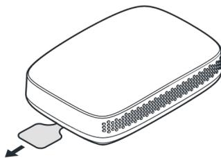
Pull the battery tab to activate the sensor
