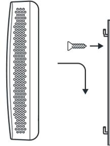
**Option 2** – Mount the sensor to the wall using a screw. If necessary, use a wall anchor.
