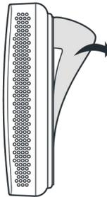
**Option 1** – Mount the sensor to the wall using the adhesive. Simply peel and stick.
