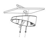
② Adjust the angle through the 3-axis adjustment structure.
