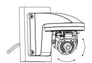
Adjust the angle through the 3-axis adjustment
