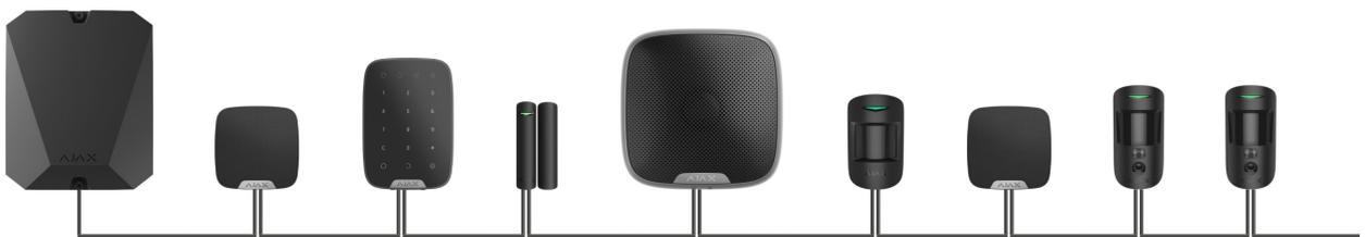
**Ring connection** occupies two bus outputs of the hub. If the ring breaks in one place, no device will be disabled. The ring reconfigures into two lines, which continue to operate normally. Users and the security company will receive notification of the break.
