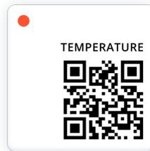
The Wireless Temperature Sensor measures the surrounding temperature and wirelessly transmits the result to a Cloud Connector (Gateway) via SecureDataShot™ technology. The Cloud Connector will relay the temperature reading to a Cloud service. The readings are performed at 15 minute heartbeat intervals. The Wireless Temperature Sensor has touch functionality for simple installation and use.
